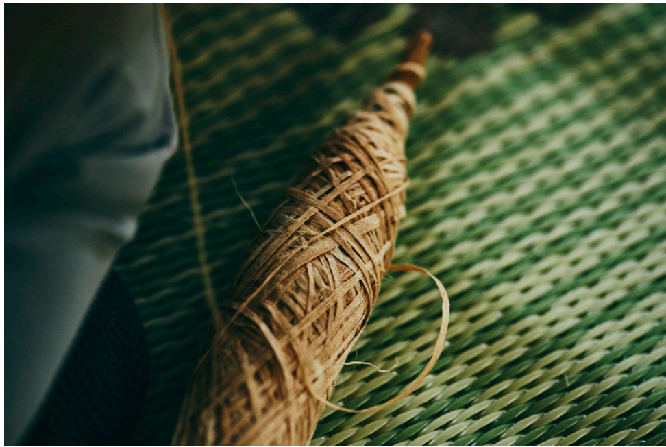
撚りをかけて紡いだ糸を糸玉にして保管し、機支度にとりかかる。 緯糸として使う糸は棒（アファンカニ）に巻き付けておく。 After twisted, spun and rolled up into a ball, the thread is put aside as the preparations of the loom begins. The thread to be used as weft is wound around a post called ahunkani .
