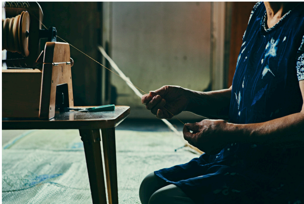
撚り加減が均一になるよう、指で調整しながら撚り機に通す。 帯一本分の糸を作るには、熟練者でも一ヶ月はかかるという。 Passing the thread through the yarn twister while adjusting it with fingers so that the tension remains even. It takes even a skilled weaver a month to produce enough threads for one obi.
