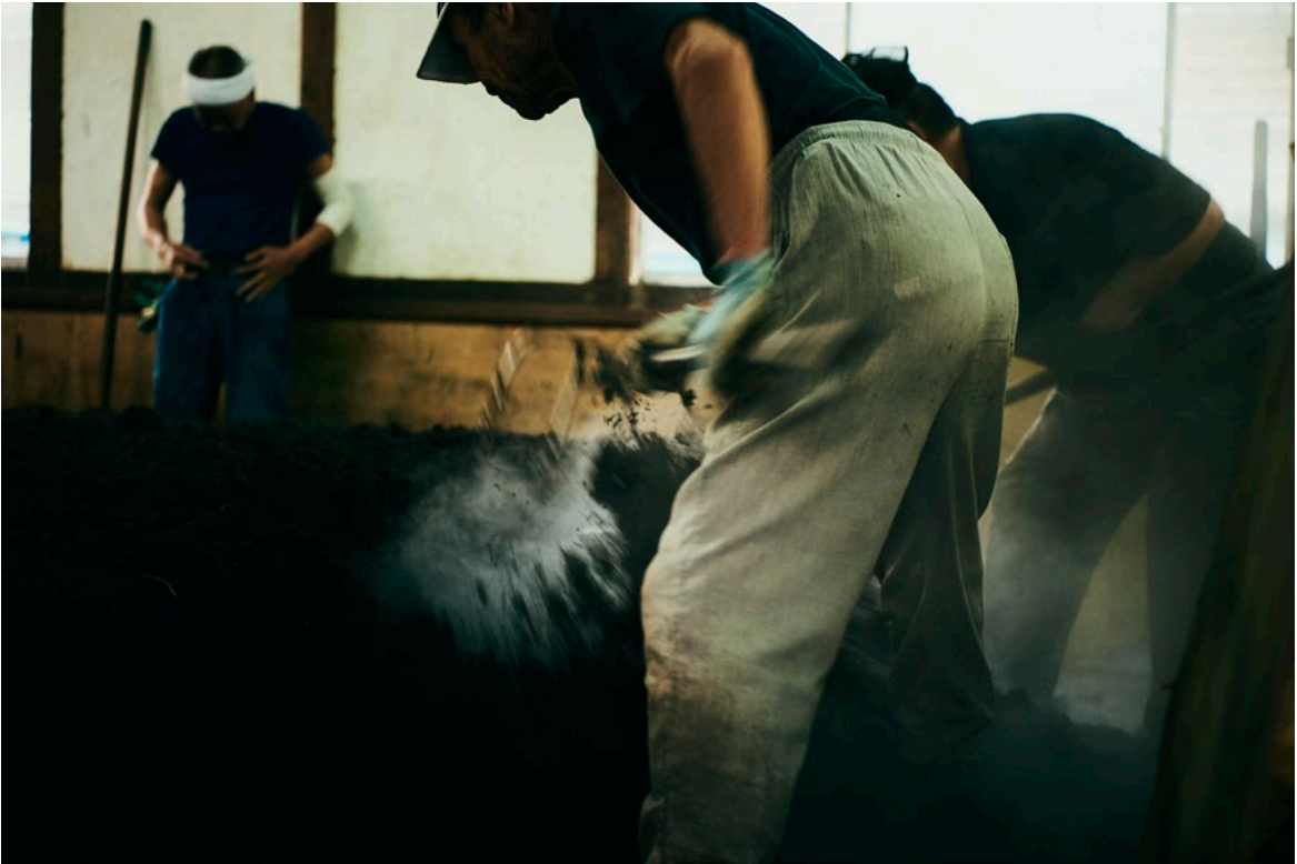
葉藍を発酵させることを、阿波では「寝さす」と言い習わし、薬づくりのために葉藍を寝さす場所を「寝床」と呼ぶ。寝床に最初の葉藍を入れる「寝せ込み」は、9月上旬の大安の日を選んで行われる。葉藍はその後、熱とアンモニアを放出しながら発酵が続けるが、5日ごとに水をかけ、木製の熊手で底から混ぜ返す「切り返し」という作業を行う。切り返した後は、元の高さ（1m程度）に納めるが、水の量、積む高さなどで薬の出来の良し悪しが決まると言われ、水を打ち管理を担当する人を特に「水師」と呼ぶ。 In Awa, to describe the fermenting of indigo leaves, they use the term nesasu (make them sleep), and the place the indigo leaves “sleep” to turn into sukumo is called nedoko ( bed ). The process of putting the first indigo leaves into nedoko , nesekomi , is conducted on Taian (the luckiest day in the Japanese calendar) in early September. The leaves continue to ferment, releasing heat and ammonia. Every fifth day, they are watered and turned over using a wooden rake. The process is called kirikaeshi . After kirikaeshi , the leaves are stored at the original height (about one meter). The amount of water and the height of the pile are said to determine the quality of sukumo , and the person in charge of watering and managing the pile is called mizu-shi (water master).
