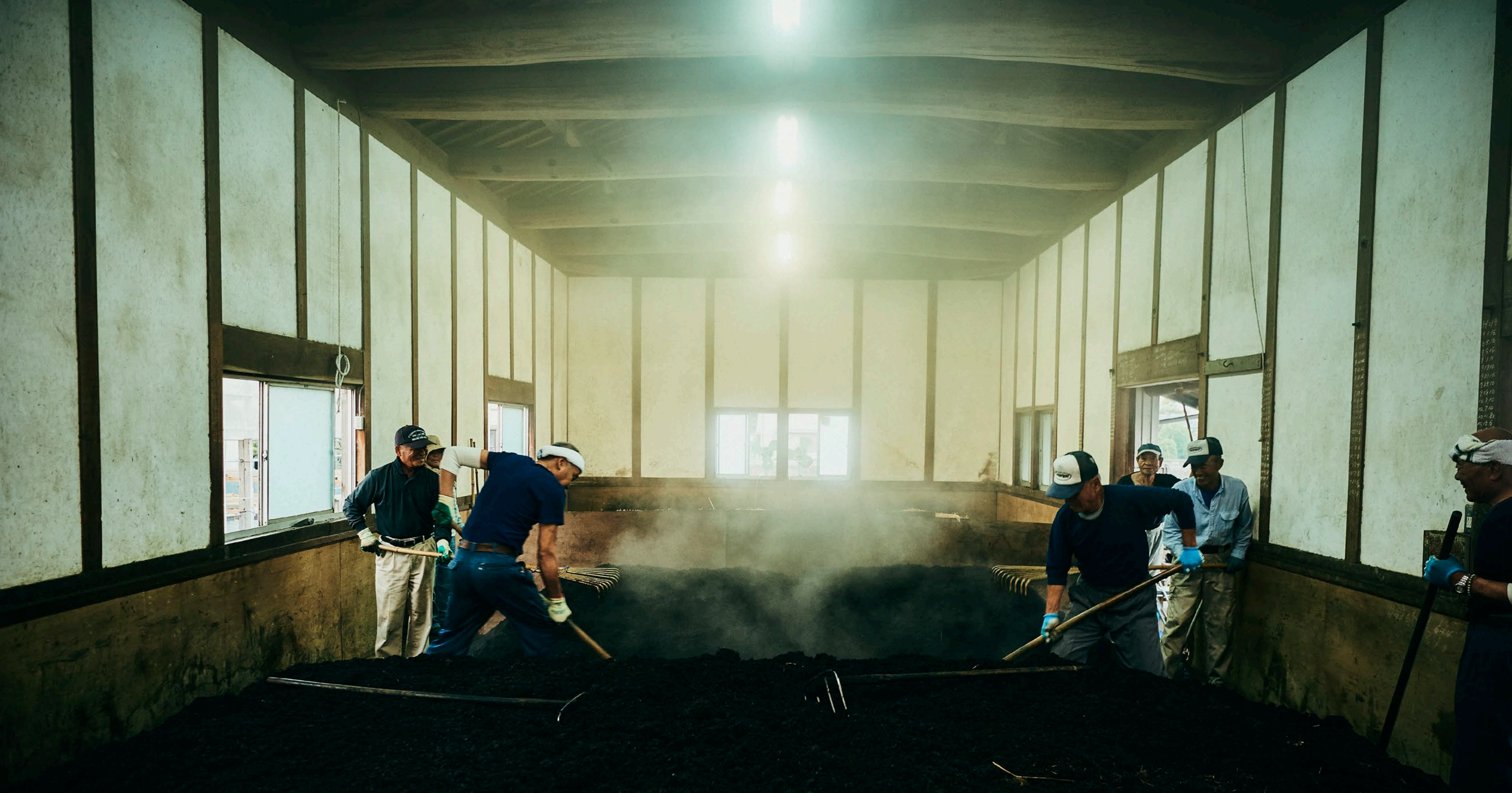
染造りのすべてに責任を持つ藍師の指令の下、切り返された葉藍が台形になって積まれ、ならされていく。発酵が進んだ葉藍は70度程度まで熱を発し、アンモニア臭も強まっていく。粘りが出でかたまりができるのを切り返しによっていねいにほぐしていく。 Under the direction of ai-shi , who is responsible for all aspects of making sukumo , the turned-over indigo leaves are piled up in a trapezoidal shape and then leveled. As fermentation progresses, the leaves heat up to about 70 degrees Celsius, and the smell of ammonia intensifies. As the leaves become sticky and clumpy, they need to be carefully loosened by kirikaeshi .
